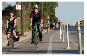
A **buffered bike lane** is a bike lane that in addition to the bike lane characteristics listed above is further separated from motor vehicle traffic with a painted buffer 1-3 feet wide (see demonstration project above).
