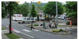
with high-speed or high-volume traffic. They may be located midblock to avoid vehicle turning movements or to provide crossings in areas where infrequent intersections create substantial out-of-direction pedestrian or bike travel. Midblock crossings should be paired with traffic-control devices such as RRFBs, lighted flashing signs and refuge islands.
